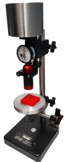
Compatible Deadweight Durometer Test Stand Model 479
