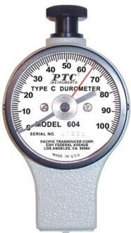
Model 604 Ergo Style Analog Asker C Durometer with 0 to 100 point dial and 1" x 1" base.
